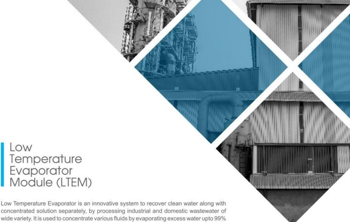
depending on Boiling Point Elevation (BPE) of fluid. All excess water is recovered as clean water or condensate separately along with concentrated fluid.
